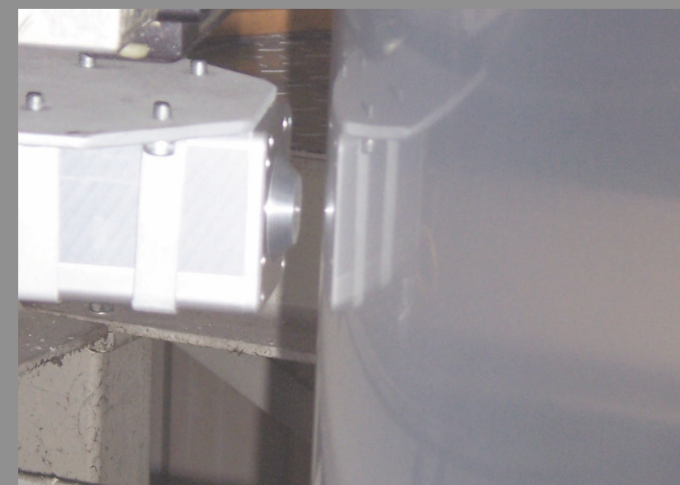
StraDex f2 - 300 sensor on an annular traverse for film production on a blown-film line.
