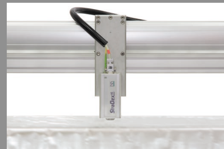
Traversing measuring unit and a StraDex sensor head. Reflection mode measurement has the added advantage that there is no need for a second traversing system on the other side of the web.
